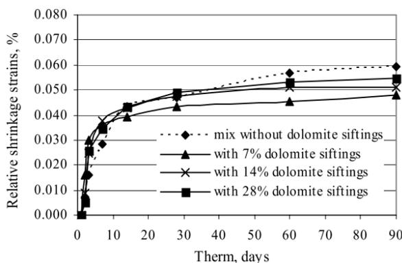
**Figure 5.** Development of concrete shrinkage strains as a function of the amount of replaced aggregates by dolomite siftings [47].
