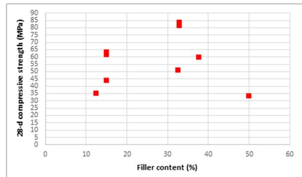
**Figure 4.** Analysis of 28-day compressive strength data from literature as a function of the dolomite filler content as a percentage of the total powder content.
