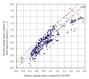
**Figure 7.** Relationship between the thermal cracking indexes of wall structures obtained by the multi-regression equation and those obtained by the 3D FEM
