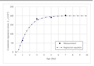
Figure 11. Restraint expansion test.
