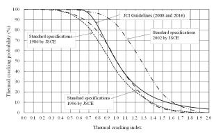
Figure 6. Thermal cracking probability.
