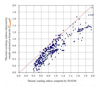
**Figure 8.** Thermal cracking indexes obtained by the simple estimation formula plotted against results of 3-D-FEM.
