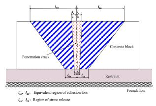
**Figure 4.** Outline of the analysis model in the CP crack width method.
