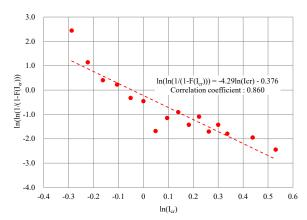
**Figure 5.** Relationship between thermal cracking index and thermal cracking probability.
