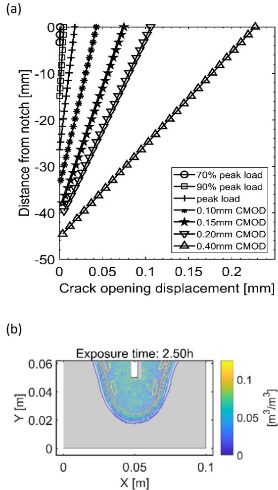
**Figure 3.** (a) Estimated crack profiles using cracked hinge model [33-35] for WST specimens investigated in [30] and (b) experimental and modelled ingress results for 0.1 mm CMOD WST specimen after exposure to liquid water. Please note: color bar indicates (measured and modelled) moisture content in m<sup>3</sup>/m<sup>3</sup>. After [31].
