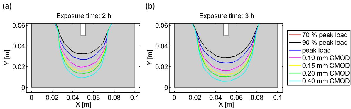
**Figure 4.** Numerical predictions of extend of moisture ingress for loaded/cracked WST specimens at selected times after exposure to liquid water. Estimated crack lengths can be deduced from Fig. 3a as the distance from notch to where COD=0. After [31].
