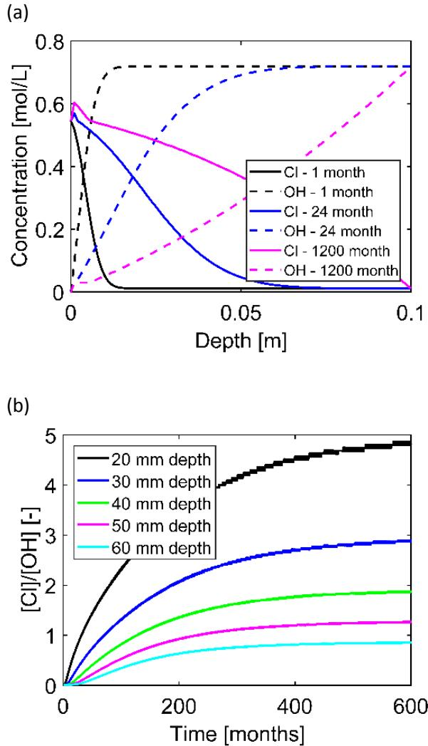
**Figure 2.** Predicted (a) chloride ion ( $\text{Cl}^-$ ) and hydroxyl ( $\text{OH}^-$ ) ion concentration as a function of depth from exposed surface after 1, 24 and 1200 month marine exposure, and (b)  $[\text{Cl}]/[\text{OH}]$  in pore solution over time.
