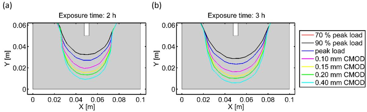
**Figure 4.** Numerical predictions of extend of moisture ingress for loaded/cracked WST specimens at selected times after exposure to liquid water. Estimated crack lengths can be deduced from Fig. 3a as the distance from notch to where COD=0. After [31].
