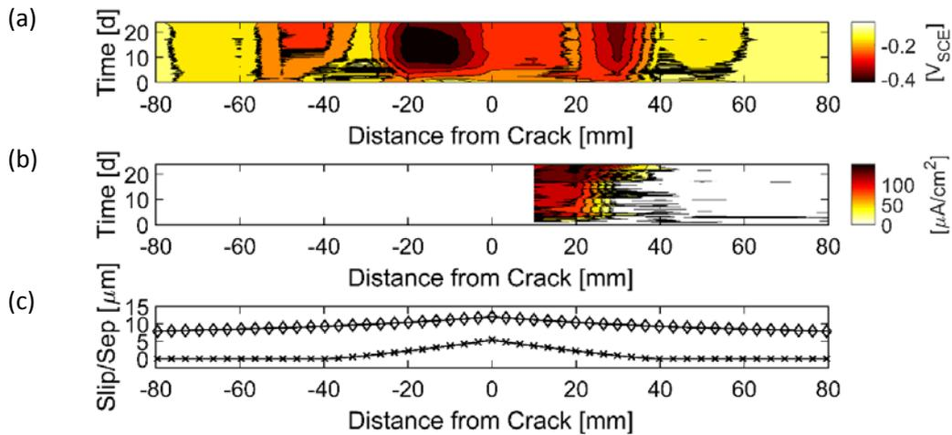
**Figure 5.** Location and time-dependent (a) open circuit potential, (b) corrosion current density (bottom), and (c) interfacial damage for specimen with crack width of 0.07 mm. After [39].
