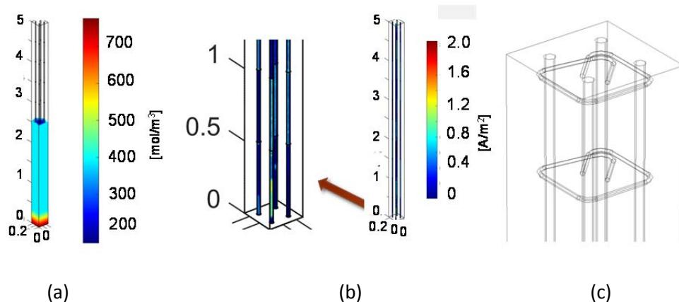
**Figure 12.** 3D prediction for an un-cracked beam of (a) free chloride concentration at the reinforcement surface, (b) absolute corrosion current density, and (c) rebar cage geometry.
