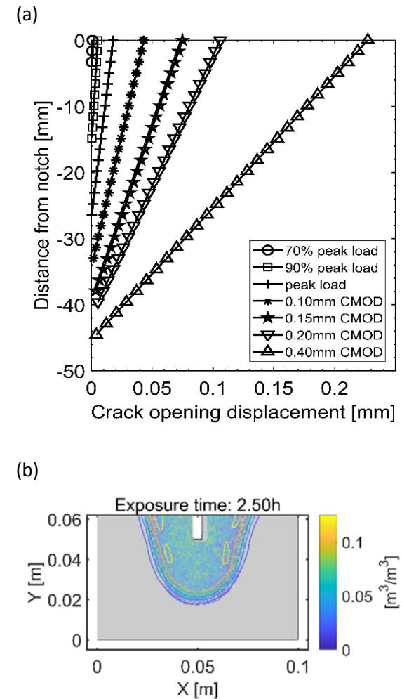
**Figure 3.** (a) Estimated crack profiles using cracked hinge model [33-35] for WST specimens investigated in [30] and (b) experimental and modelled ingress results for 0.1 mm CMOD WST specimen after exposure to liquid water. Please note: color bar indicates (measured and modelled) moisture content in  $\text{m}^3/\text{m}^3$ . After [31].
