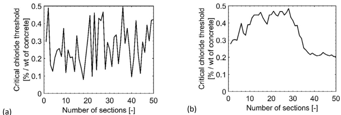
**Figure 8.** Distribution of initial chloride threshold values along the length of a single rebar. (a) using a random distribution, and (b) using a more realistic, multi-variate uniform random distribution.
