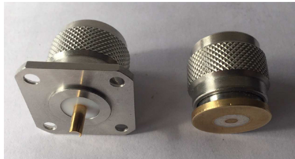
Figure 3. N connector (left) and the derived open-ended coaxial probe (right).
