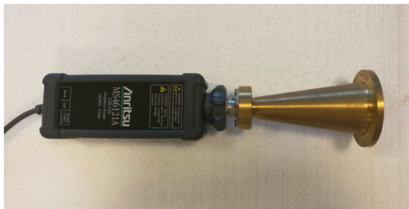
Figure 1. Open-ended coaxial probe and VNA used during the experiments.
