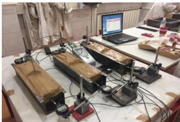
Figure 6. Testing autogenous deformations.
