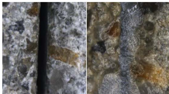
Figure 2. Micrographs of a self-healing (containing bacterial ACDC granules) mortar specimen with 300 \mu\text{m} wide crack before (left) and after (right) 28 d submersion in a 0.4 M chloride solution, showing complete crack healing (courtesy of Yusuf Çağatay Erşan).
