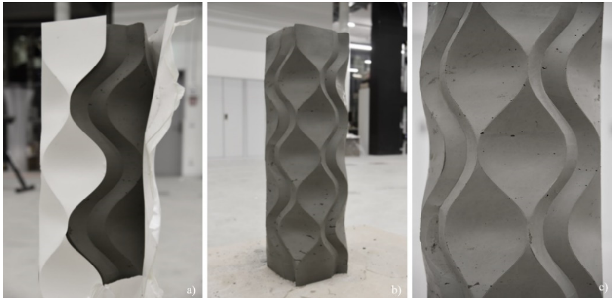
Figure 6. a) demoulding the 1-meter-tall concrete column prototype after 4 hours. b) demoulded column. c) close-up showing the suboptimal surface quality.
