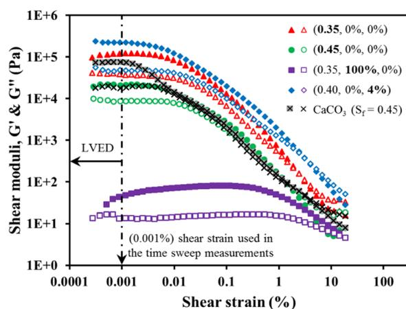
**Figure 5.** Variations of shear moduli with shear strain between 0.0001% and 20% and at angular frequency of 10 rad/s. ( $G'$ : full symbol,  $G''$ : empty symbol), the two % values indicate the HRWR and silica fume percentages. Reproduced with permission from [17].
