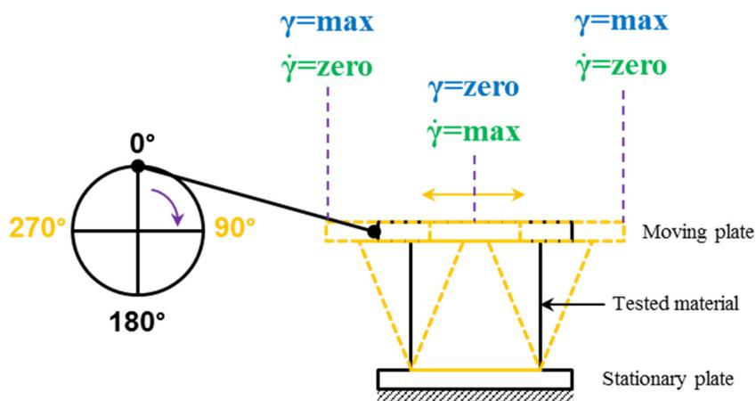
Figure 2. The two-plates-model and oscillatory shear, adapted from [3].
