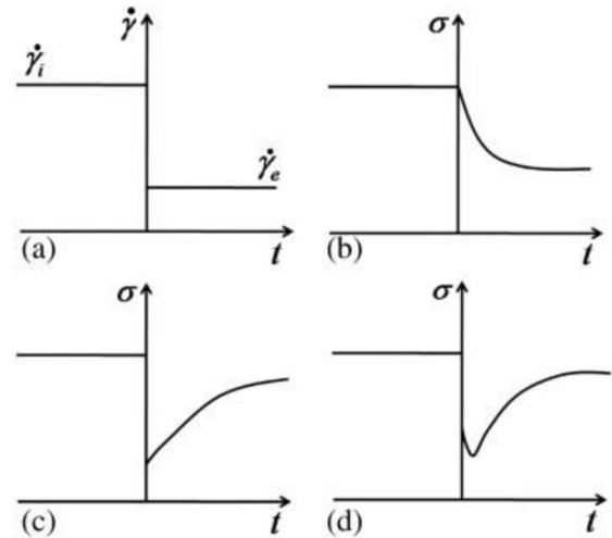
**Figure 3.** Responses to a sudden reduction in shear rate (a): b) viscoelastic; c) inelastic thixotropic; d) most general. Reproduced with permission from [20].
