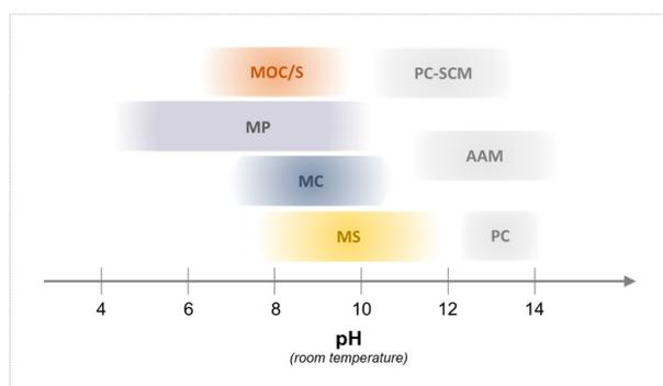
**Figure 2.** Approx. pH range for the stability of different MgO-based cement systems. MOC/S = Mg-oxysulfate / Mg-oxychloride cements, MC = Mg-carbonate cements, MP = Mg-phosphate cements, MS = Magnesium silicate cements, PC-SCM = blended Portland cements, AAM = Alkali activated materials, PC = Portland cement.
