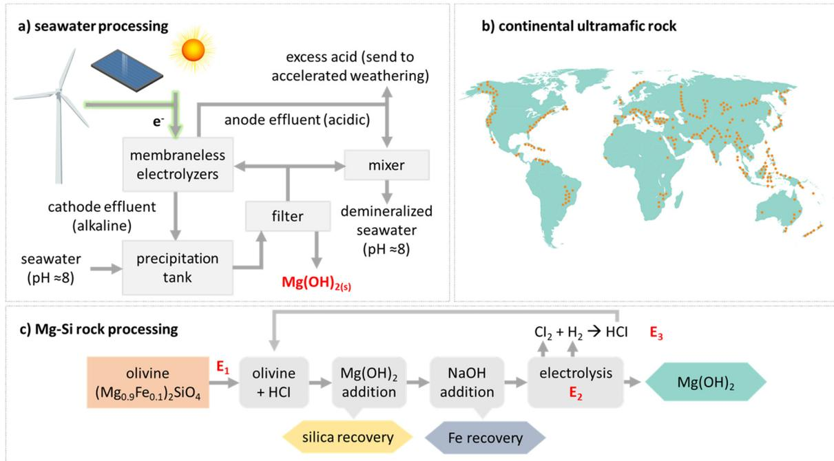
**Figure 1.** a) Currently known worldwide distribution of ultramafic rock (adapted from [23]); b) Process routes for Mg extraction from seawater (adapted from [14]); c) Process (acid) route for Mg extraction from silicates (adapted from [23]).
