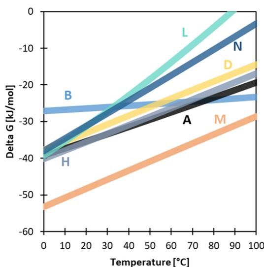
**Figure 3.** Free energies relative to MgO in kJ/mol as a function of temperature at pCO<sub>2</sub> = 0.4 mbar and saturated vapour pressure for different HMC. A: artinite, D: dypingite. H: hydromagnesite, L: lansfordite, M: magnesite, N: nesquehonite. Calculated based on the thermodynamic data compiled in [104].
