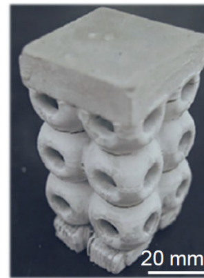
Fig. 12. Cellular architected (Schwarzite) cementitious-polymer composites [104].
