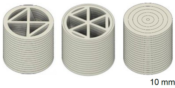
Fig. 8. Architected MgO binders with cellular and solid architecture [90].
