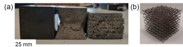
Fig. 11. (a) undeformed specimen (left) compared with deformed unconfined (middle) and confined specimen (right) and (b) 3D-printed steel auxetic lattice [102].
