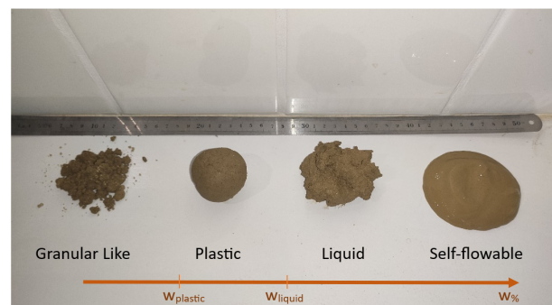
Figure 2: Possible earth consistencies of a same earthen material with increasing water content in relation with the Atterberg consistency limits commonly used in geotechnics.
