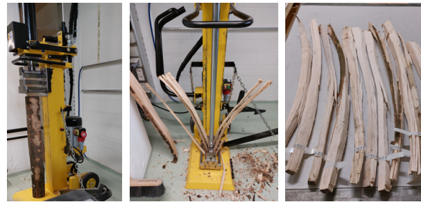
Figure 1. Splitting process in a conventional splitting machine with a modified, multi-blade splitting head resulting in split rods for further processing.
