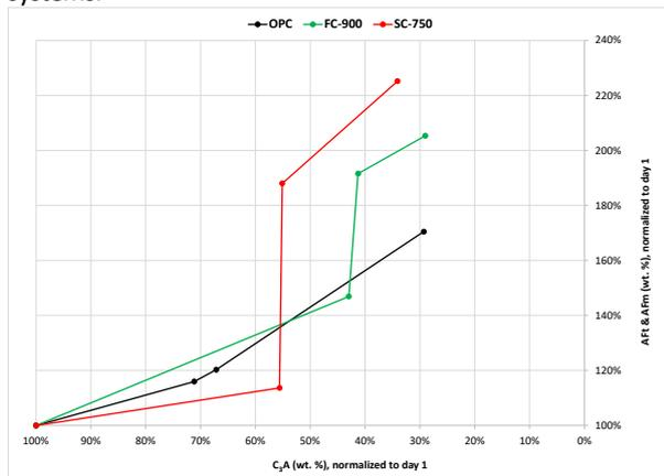
Figure 10. Aft, AFm and C<sub>3</sub>A content at 1, 3, 7 and 28 days, normalized by its respective content at 1 day.
