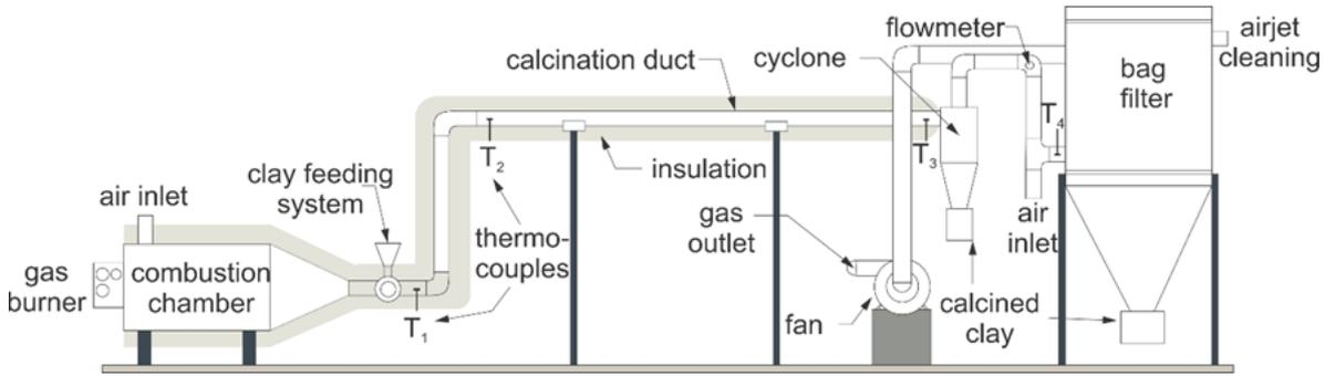
Figure 1. Diagram of the Clay Activation Unit.
