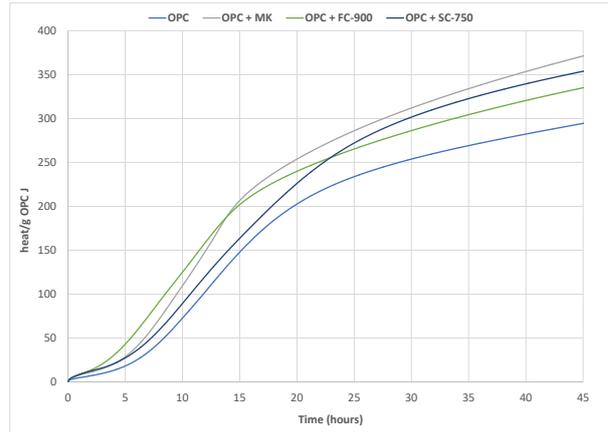
Figure 7. Cumulative heat of hydration cement pastes.
