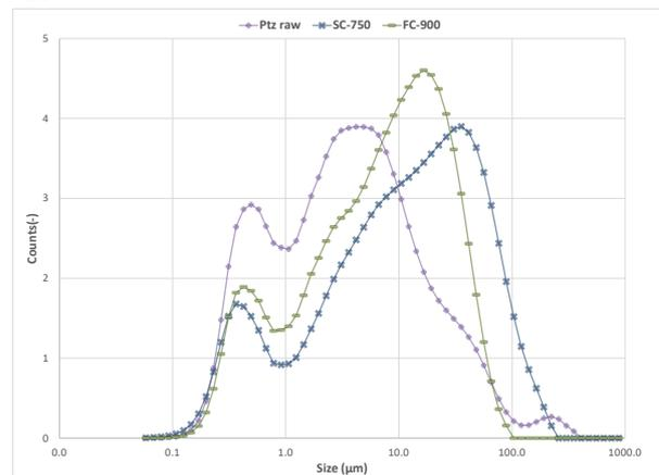
**Figure 4.** Particle size distribution of the calcined material vs. raw clay.
