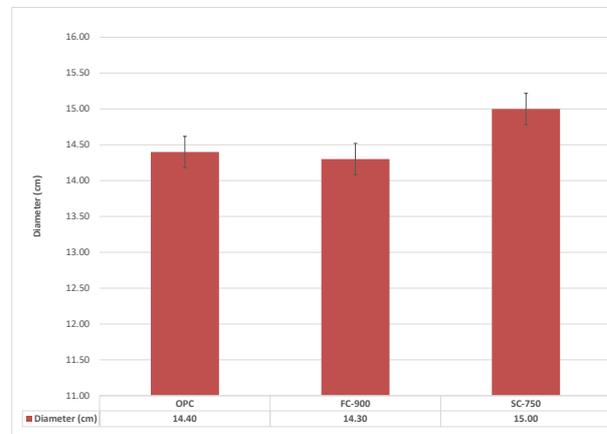
Figure 11. Spread in standard mortars.
