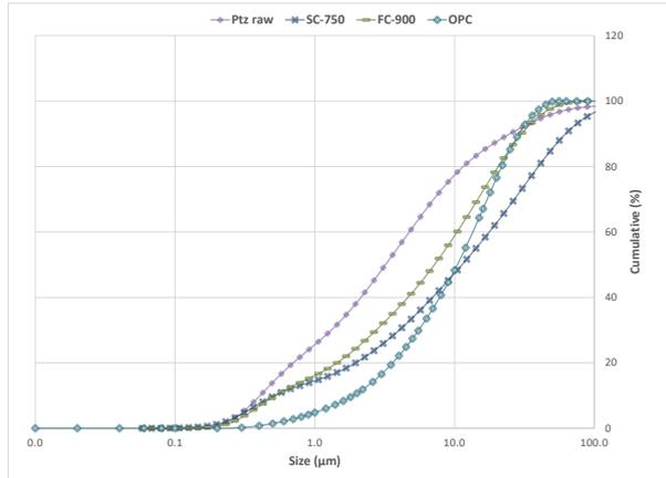
Figure 5. PSD of the different materials.
