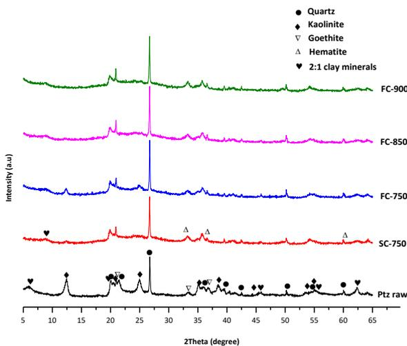
**Figure 3.** XRD of the calcined material.
