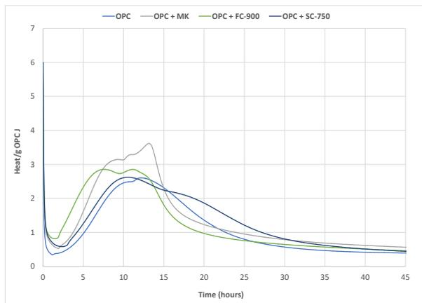
Figure 6. Heat of hydration cement pastes.
