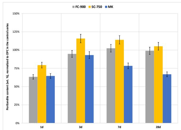
Figure 8. CH consumption on cement pastes.
