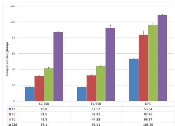
Figure 12. Compressive strength in standard mortars
