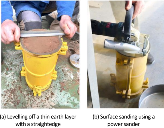
Figure 2. Methodology for obtaining a clean and parallel surface.
