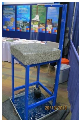
Figure 3. Water infiltration in PCPC.
