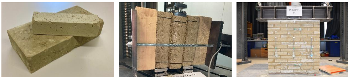
Figure 1. Test specimen samples (left to right): masonry components, three-block-specimen, and masonry.
