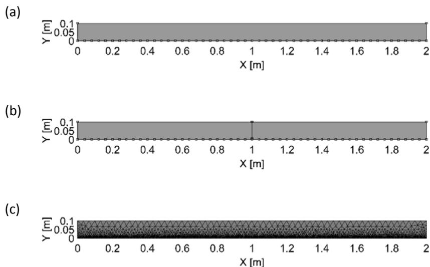
**Figure 9.** Lattice model geometry for (a) un-cracked beam, (b) cracked beam, and (c) mesh. After [46].
