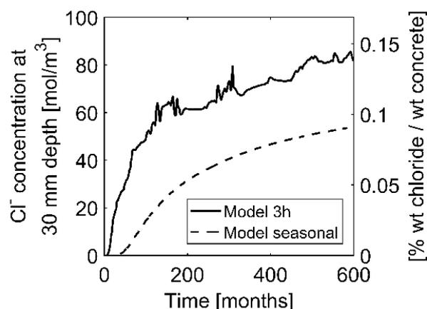
**Figure 1.** Prediction of chloride concentration at 30 mm depth over 50 years using a coupled heat and mass transport model applying detailed meteorological data (per 3 h) or averaged seasonal data. After [19].
