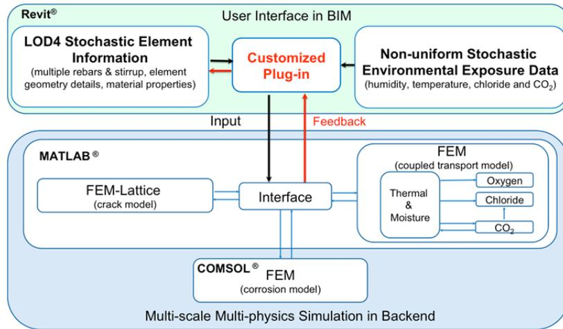
**Figure 7.** Architecture of the multi-physics and multi-scale model to predict and assess the deterioration of reinforced concrete structures in an interactive framework using a customized plug-in to connect the deterioration model to a user-friendly building information modelling (BIM) interface [40].
