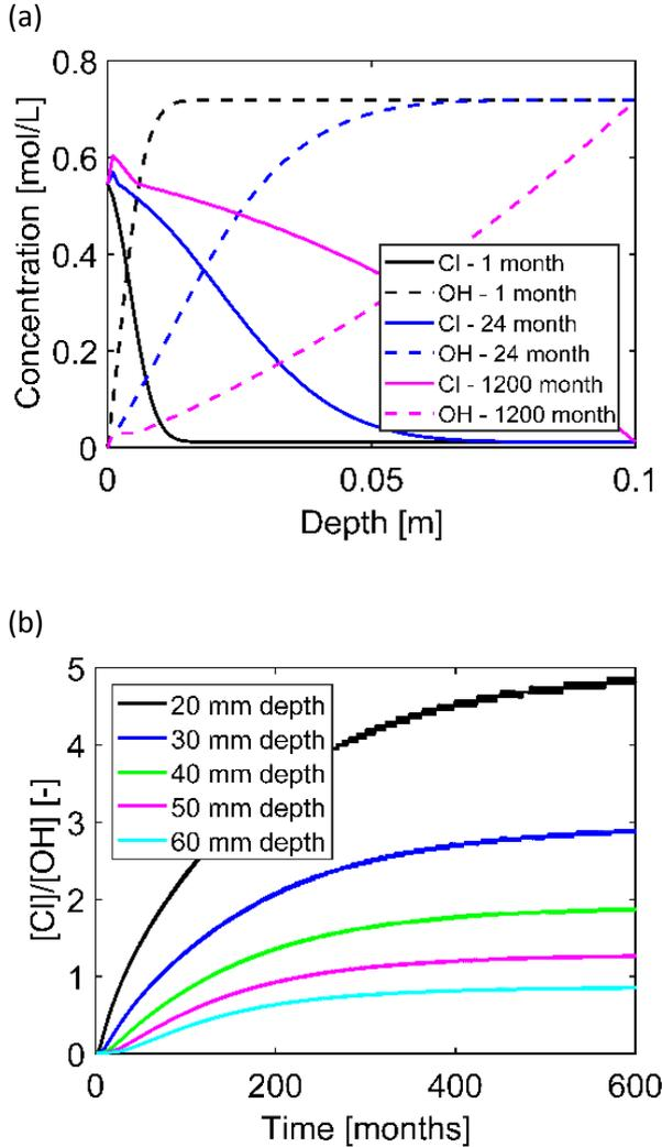
**Figure 2.** Predicted (a) chloride ion (Cl<sup>-</sup>) and hydroxyl (OH<sup>-</sup>) ion concentration as a function of depth from exposed surface after 1, 24 and 1200 month marine exposure, and (b) [Cl<sup>-</sup>]/[OH<sup>-</sup>] in pore solution for selected depths over time.
