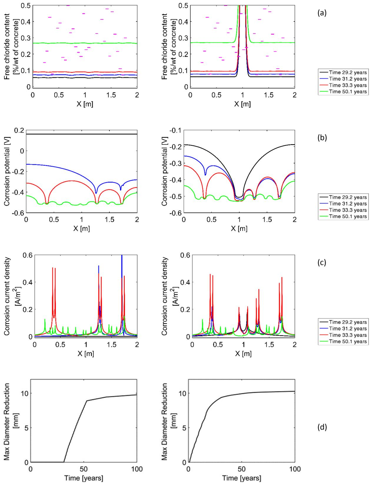
**Figure 11.** 2D prediction for an un-cracked (left) and a cracked beam (right) with geometry as shown in Fig. 9 of (a) chloride threshold (purple lines) and free chloride concentration at the reinforcement surface, (b) corrosion potential, (c) absolute corrosion current density, and (d) maximal rebar diameter reduction. After [46].
