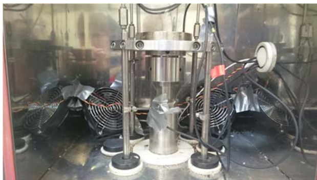
Figure 7. Improved, improved setup to increase air flow velocity in the 2003 device.
