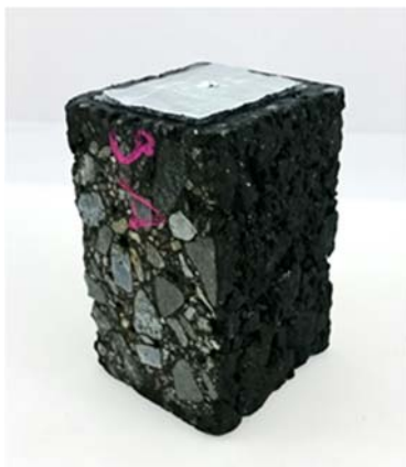
Figure 4. Schematic view and photo of a dummy specimen.
