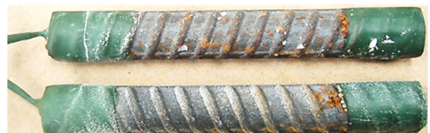
Figure 4. An example of before and after testing for pitting potential is shown at the top of the figure. The after tested bar showed clear pitting corrosion underneath the side rib with no crevice corrosion underneath the lacquer. Bars at the bottom, tested for similar purpose but showed crevice corrosion, albeit pitting corrosion in some case, were discarded.
