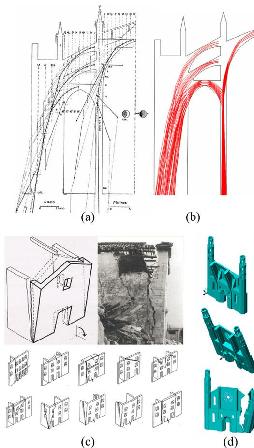
**Figure 10.** Mallorca cathedral: (a) Thrust line application from Rubió, 1912; (b) numerous alternative thrust lines, from analytical calculations [24]. Kinematic analyses: (c) an abacus of out-of-plane overturning modes [25]; (d) definition of collapse mechanisms for the façade of Santa Maria del Mar church in Barcelona [10].
