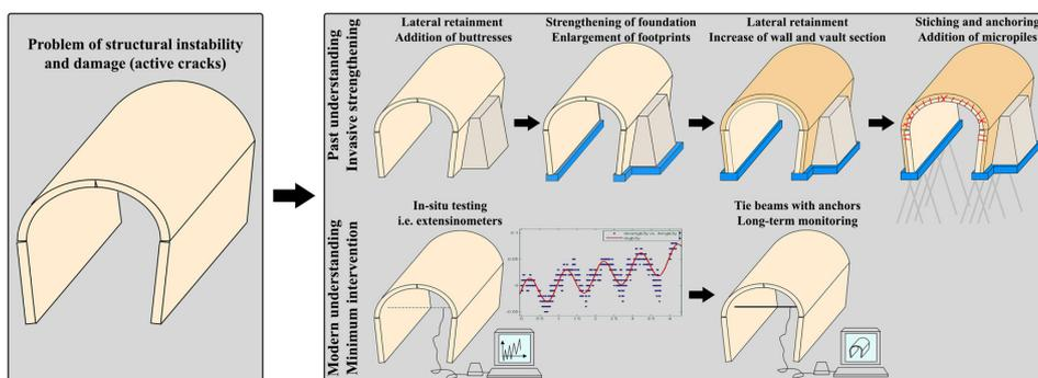
**Figure1.** Conservation and intervention. Blind confidence in modern and invasive techniques, with loss in authenticity and mistrust on the original capacity of the ancient structure vs. the modern understanding, combining minimum interventions and long-term monitoring.
