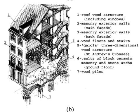
Figure 4. Lisbon earthquake 1755: (a) representation of the tsunami and fire, after the earthquake, from a German engraving [5]; (b) perspective drawing of a typical ‘Pombalino’ building, post to the earthquake [6].
