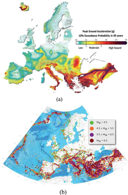
Figure 3. Seismic activity in Europe: (a) European seismic hazard map of 2013; (b) historical earthquake database for the period of 1000 to 2007 AD, with a magnitude range  $1.7 \leq M_w \leq 8.5$  for Europe, Central and Eastern Turkey, as compiled in the SHARE European Earthquake Catalogue (SHEEC) [4].
