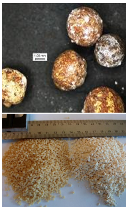
Figure 3. First generation expanded clay based healing agent (top image) and next generation lactate-derivative based healing agent (bottom image).
